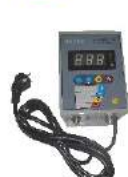
Digital pressure gauge box
