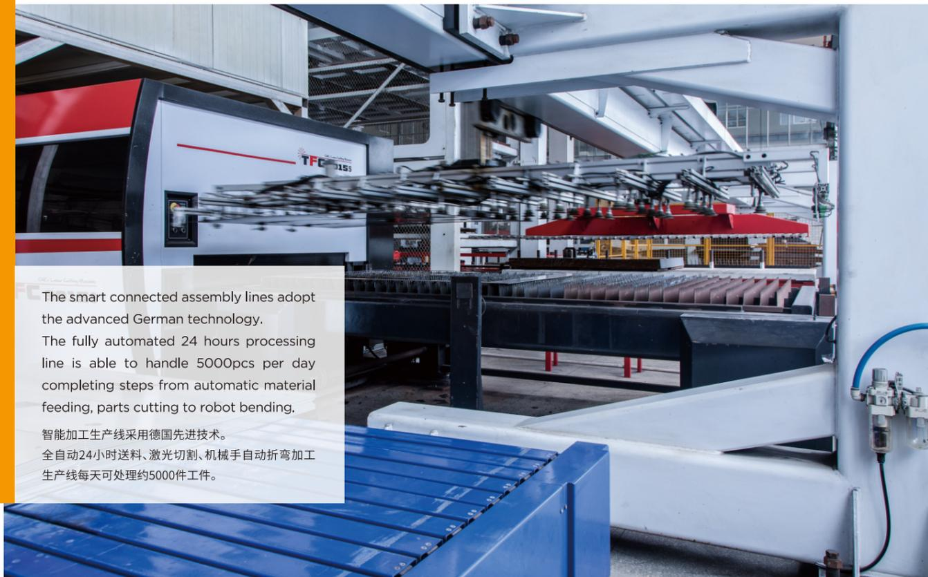
The smart connected assembly lines adopt the advanced German technology. The fully automated 24 hours processing line is able to handle 5000pcs per day completing steps from automatic material feeding, parts cutting to robot bending.
