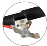
Foot pedal for the pneumatic wheel clamp
