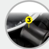
Nylon bead roller leaves no mark on rim and makes tyre changing easier.
