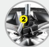
Quick clamping with central positioning function.
