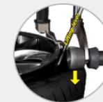
Pressing roller assists in preventing rim scratch 压胎滚轮防止轮毂因刮蹭受损。
