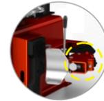
The bead breaker is adjustable in four positions. 压胎铲可向四个方向调节。
