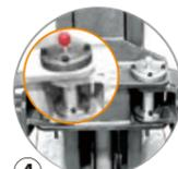
④ Arm lock engaged automatically when lifting
