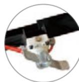
Foot pedal for the pneumatic wheel clamp
