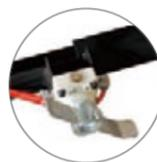
Foot pedal for the pneumatic wheel clamp
