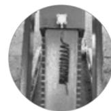
Precision machined double sided safety teeth design 独特双边安全锁齿设计
