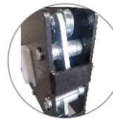
Equipped with main insurance and rope break insurance on each column 每个立柱设有主保险和 断绳保险
